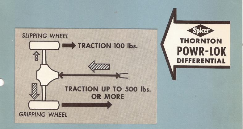
Under the same conditions the Thornton POWR-LOK differential applies many times the driving force of the curb wheel to the wheel on the street with the better traction and the vehicle starts normally.
